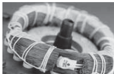
Fig. 47 Thermal switch incorporated in windings
