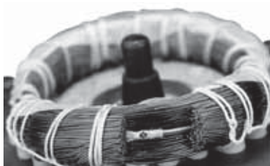
Fig. 45 PTC sensor incorporated in windings
